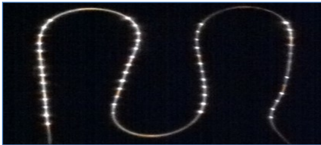
Figure 4: Illuminated Fibre highlighting Periodic Grooves
