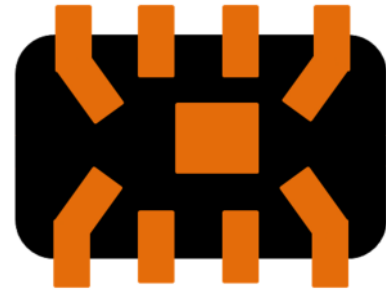
Figure 2. Schematic of the internal structure of the integrated circuit showing the 8 pins and the microelectronic circuit chip in the middle.
