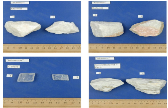
Figure 2 Mineral samples. Marble (a), dolomite (b), calcite (c) and calcite/dolomite + pyrite (d)
