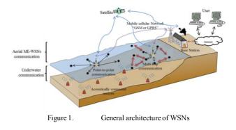
c) Underwater Sensor Networks with autonomous underwater vehicles: Autonomous Underwater Vehicles (AUVs) are used to enhance the capabilities of underwater sensor networks in terms of self-configuration of sensor nodes,(e.g. maintenance of underwater network infrastructure), adaptive sampling, power supply issues and depth capability which can reach up to 1500m. Furthermore, global position satellite (GPS) technology can be used to track the location of the vehicles on or near the surface.
