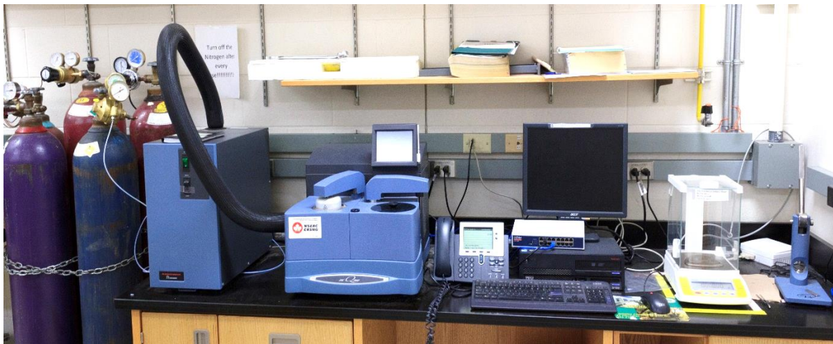
Fig. 3.1. Photo of a modulated differential scanning calorimetry system manufactured by TA instruments.
