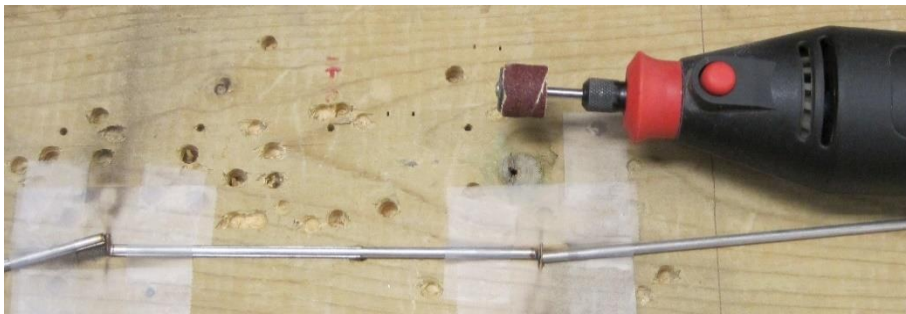
Fig. A.1 Stainless steel needles have been cut and the cut off tool with a sandpaper tip on.
