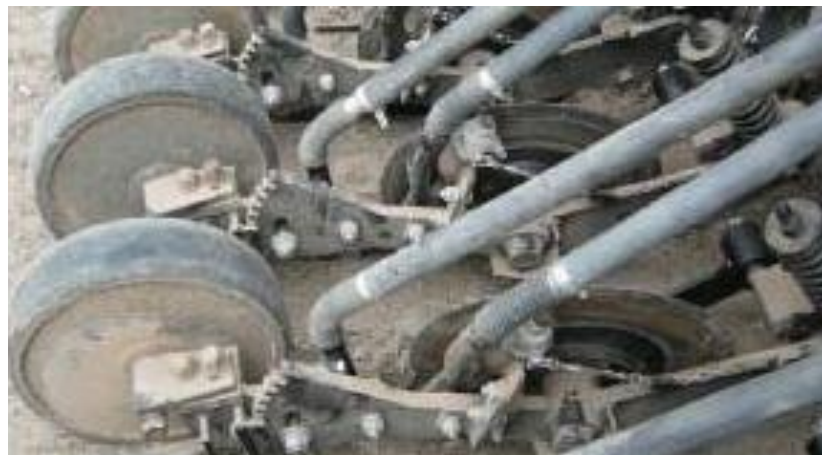
Figure 3.43. Specialty No Till (SNT) Double-Shoot System (Courtesy of Specialty No Till SNT website- http://www.specialtynotill.com.au/ ).
