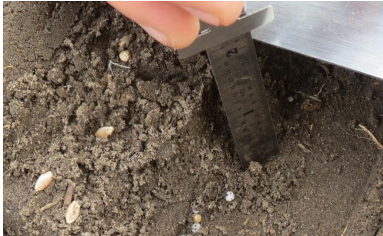
Figure 4.42. Step No. 8: Fertilizer depth measurement.
