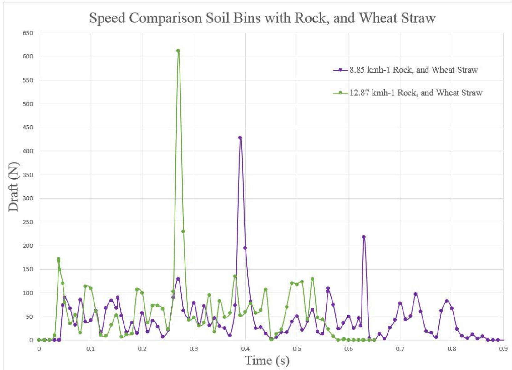
Figure G. 4. Speed Comparison Soil Bins with Rock, and Wheat Straw
