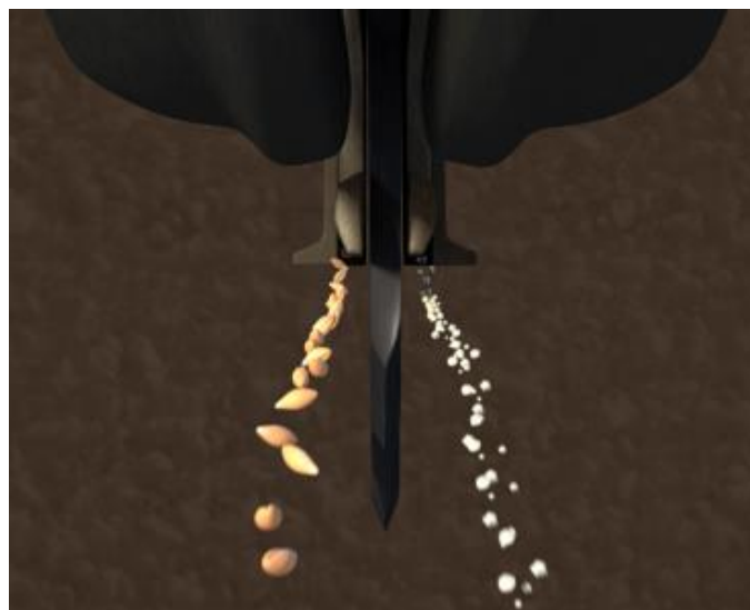
Figure 3.25. Cross Slot No-Tillage System seed and fertilizer placement (Courtesy of Cross Slot No-Tillage Systems website- http://www.crossslot.com/modules/SP_Gallery/gallery.php?gallery=1 ).
