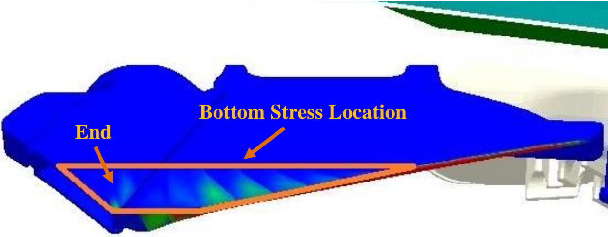
Figure 5.7. Bottom view of the knife at 8.85 km·h -1 .
