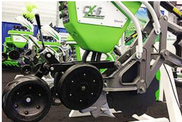
Figure 3.17. Clean Seed Capital Group Ltd. Opener assembly (Courtesy of Clean Seed Capital Group website- http://www.cleanseedcapital.com/cx-6tridenttechnology.html ).
