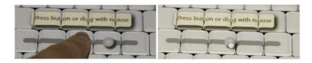
Figure 2.2.5: Touch-Display keyboard. Slider controls being displayed on the keyboard which can be manipulated using finger touch.
