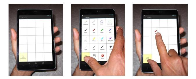
Figure 2.1.5: FastTap selection: (Left) Default state of FastTap interface, (Center) Visual search by novice user, (Right) Rapid command selection by expert user without waiting for commands to appear [75].
