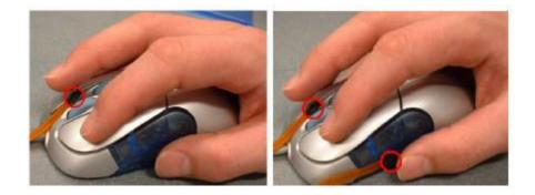
Figure 2.2.2: (Left) Uni-pressure augmented mouse with a sensor in the top location for the second finger. (Right) Dual-pressure augmented mouse with sensors located in the top location for the second finger and in the left location for the thumb [44].
