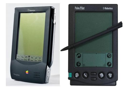
Figure 2.1.2: Pre-iPhone era devices with touchscreen interfaces. Left: Apple Newton Message Pad launched in 1993 [173]. Right: PalmPilot launched in 1992 [162].
