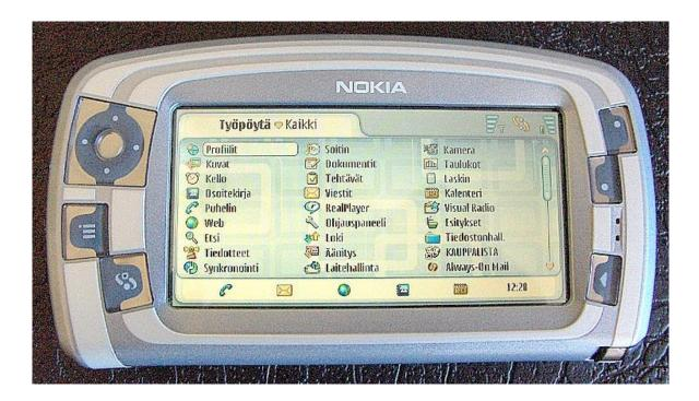
Figure 2.1.3: Nokia 7710 launched in 2004; it used resistive touchscreen technology [158].
