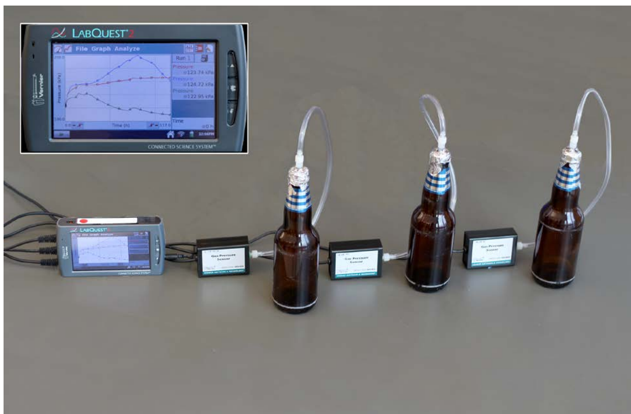
Fig. 5.1. Vernier gas pressure sensor setup.
