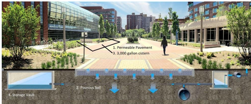
Figure 4: Existing stormwater management that can be seen in front of the Institute of Environmental Sustainability [16]
