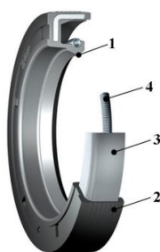
Figure 1: Radial lip seal schematic [2]
