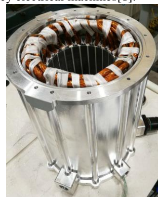
Fig. 1. Litz wire use within an aerospace generator.
