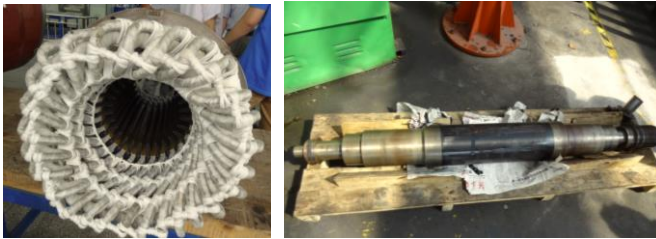
(a) Stator with windings (b) Rotor Fig. 19. Stator and rotor for high speed PMSM
