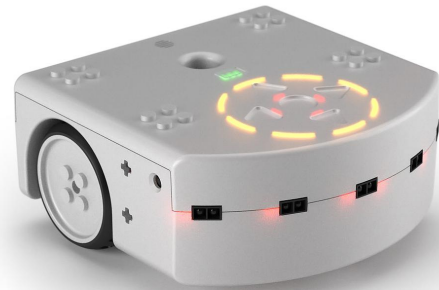
Fig. 1: The Thymio II robot (110x112x54mm).
