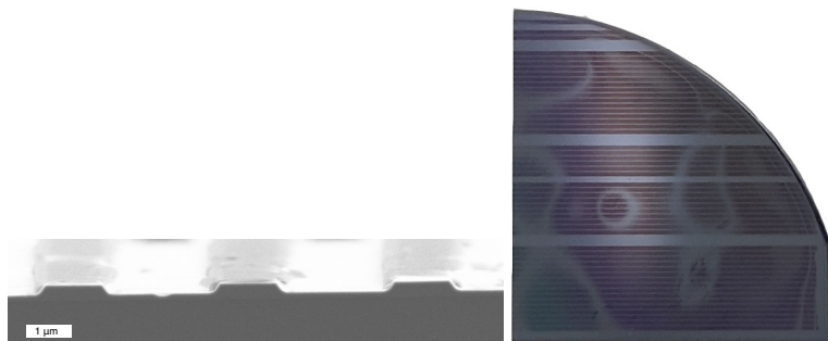
Figure 4.2: SEM pictures. a) A cross section of the grating etch. It shows the grating with an etching depth of 200 nm and a resist thickness of roughly 70 nm. b) Top view of the processed wafer, the grating was etched uniformly, indicated by the near absence of Newton's rings. Figure b) taken from Ref. [64].
