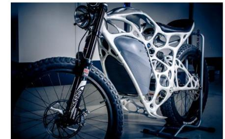
SLM-manufactured aluminium frame,
