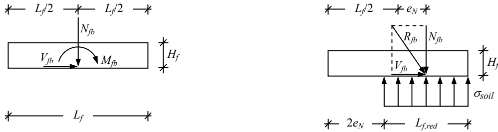
Fig. 3.40: Assumed soil pressure distribution for calculation of bearing capacity in case of eccentric vertical load
