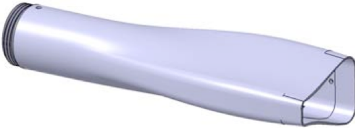
Figure 3.9 Outlet duct of the hot streak generator designed for the non-axisymmetric hot streak shape
