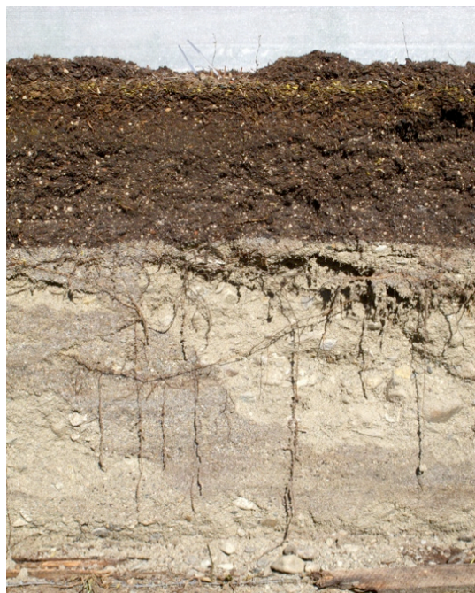
Fig 3. Soil in the mesocosms, consisting of 15 cm topsoil (humus) and 30 cm subsoil (sand and gravel).
