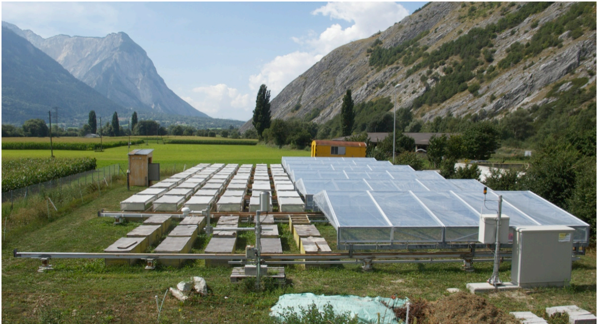
Fig 2. Experimental site near Leuk (VS, Switzerland) with mesocosms covered by white shade cloths and opened mobile rainshelters.
