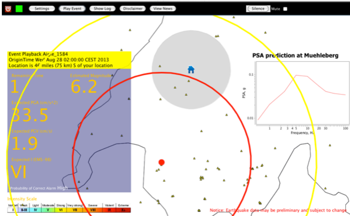
Figure 2. Example UserDisplay screenshot showing peak ground motion and response spectrum predictions at the site of Mühleberg, based on the location and local magnitude of the 1584 Aigle event. The grey-shaded area around the target is the expected blind zone. The red and yellow circles are the S- and P-wave fronts, respectively.
