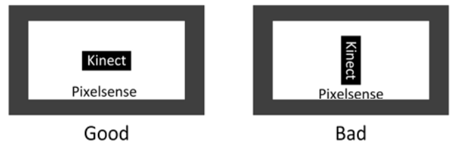
Figure 11: The long sides of Kinect and PixelSense have to be aligned for the filter to work correctly.
