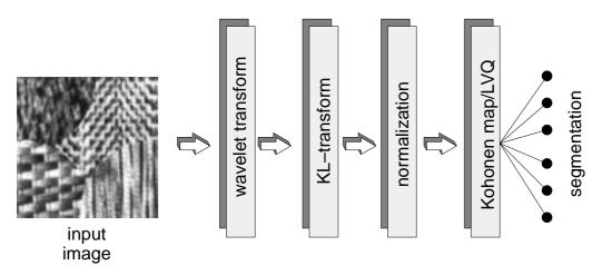
Fig. 10 Wavelet-based data analysis pipeline.
