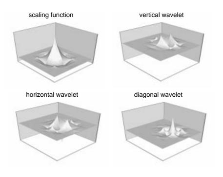
Fig. 5 2D–Coiflet wavelets and scaling function
