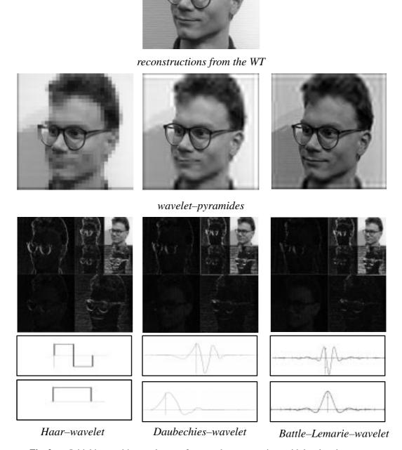
Fig. 2 Initial image, it's wavelet transforms and reconstructions with local variations of the level—of—detail for different wavelet—types
