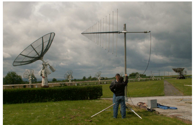
Fig. 1. Logarithmic periodic antenna at Humain station connected to Callisto spectrometer. Top right in the background an old "Würzburg Riese", remains from World War II. In the background left the East-West arm of the old solar interferometer.
