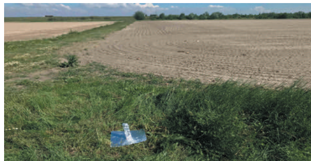
Figure 2. Example of a thermal Ground Control Point (GCP)
