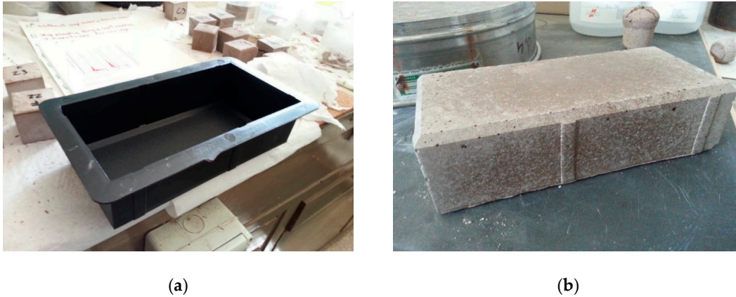
Figure 2. (a) Plastic mold; (b) Final paving blocks after de-molding.
