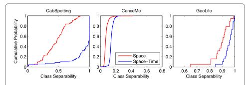
**Figure 5** Empirical CDF of the geometric separability over the three datasets. For each dataset, we show the cumulative probability (y-axis) of the per class geometrical separability (x-axis). The red line refers to the case where only the spatial information is used, whereas the blue line refers to the case in which also time is taken into account. We observe that in general the addition of the temporal dimension makes the data much easier to separate.
