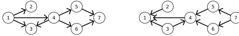
Figure 20: Different End Types. Different types of sinks (left) and sources (right) are shown. Both can be differentiated into three types. The ends that are connected only to one other vertex (vertex 2 in both graphs). The second type comprises the ends that are connected to more than one vertex, but these vertices have a specific order (vertex 3 in both graphs). The last type comprises the ends that connected to more than one vertex with unclear order (vertex 7 in both graphs).
