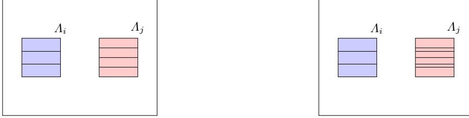
Fig. 4: Left: TBPN-splines allow to refine the subdomains A_a and A_b independently. Right: THB-splines require nested knot vectors for any pair of subdomains.
