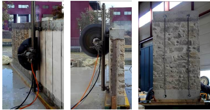
Figure 1: Saw-cutting of a long wall to obtain specimens for vertical compression tests.
