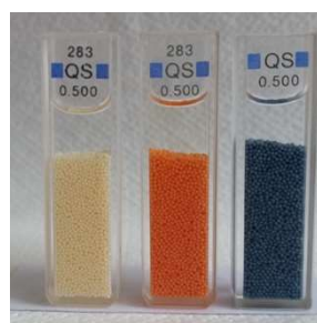
Figure 1 Cuvettes filled with suspended solid phase in HNO 3 solution. From left to right, Marathon resin, TazoC-Mar@, TazoC-Mar@ after contact with Pd(II) solution.
