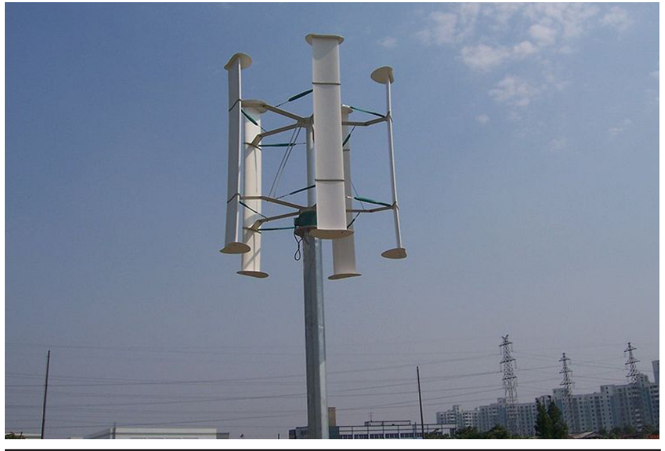
Figure 2: A Modern H-Rotor Darrieus Wind Turbine (Courtesy of Shaghai Aeolus Windpower Technology, LTD.)
