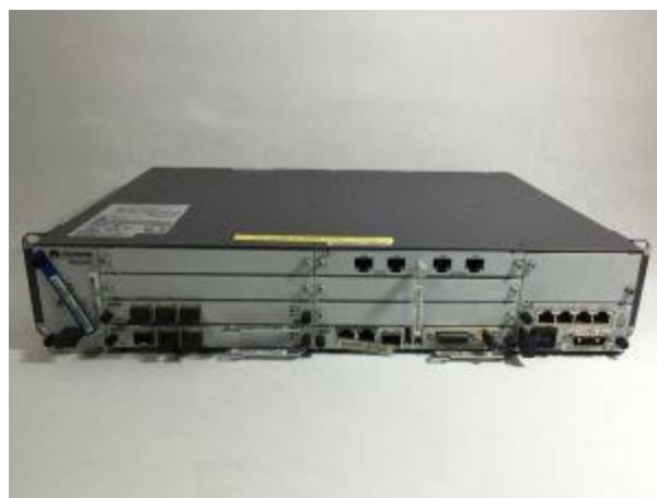
Figura 2.22 Huawei BTS3900. Huawei, (2016)
