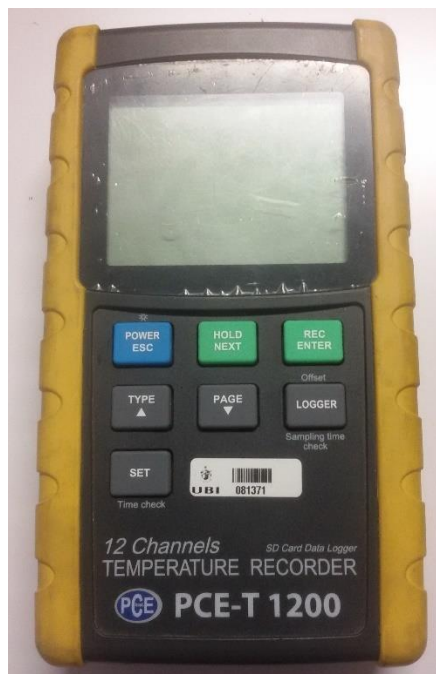
Figura 4.6 - Data logger PCE-T 1200 da PCE instruments.
