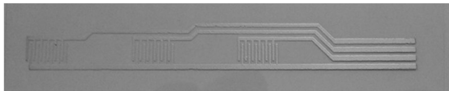
Figure 28. Sample of the polymeric matrix with printed electrodes.
