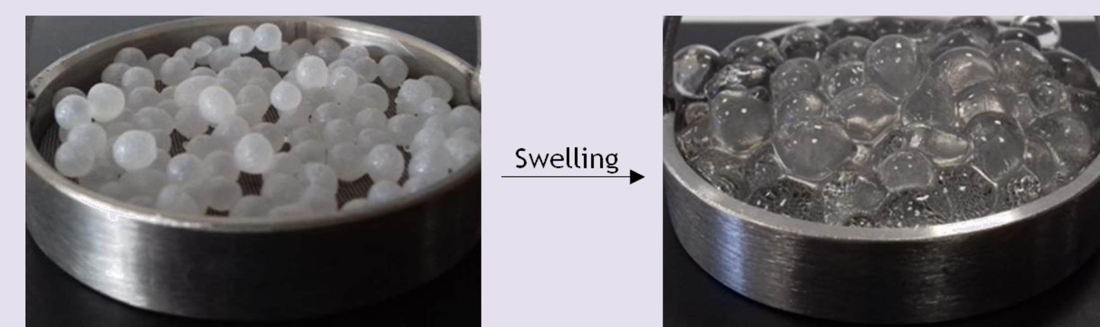
Figure 4 - DDS before (left) and after (right) the kinetic studies of Diclofenac release, resulting from the swelling of the 3D cellulose based polymeric matrix.
