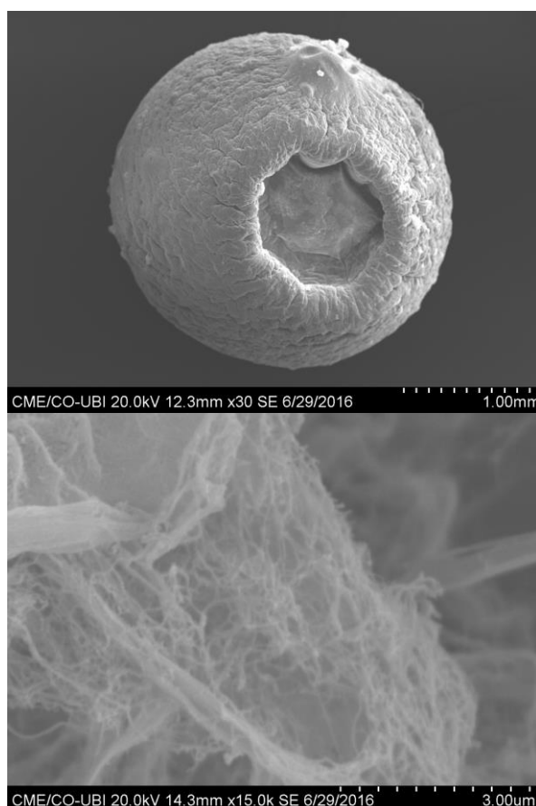
Figure 1. a) SEM image of DDS made from NFC (30X). b) SEM image of NFC structure inside the DDS (15000X)
