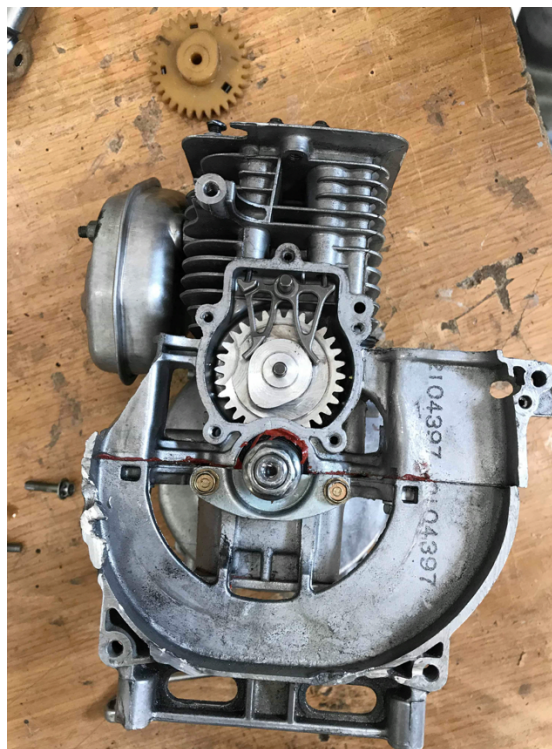
Figure E.2 - Aluminium cam installed in the Honda GX31 and, in the upper-right corner, the original Honda GX31 cam.
