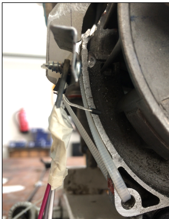
Figure H.7 - Detail of the Hall effect sensor in place, in order to read the magnetic pulses of the flywheel magnets during the test runs.
