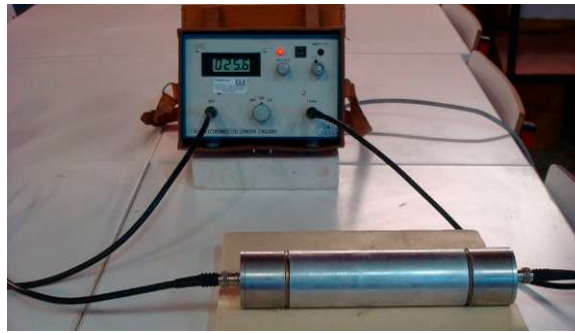
Figure 8. Calibration of the PUNDIT apparatus.
