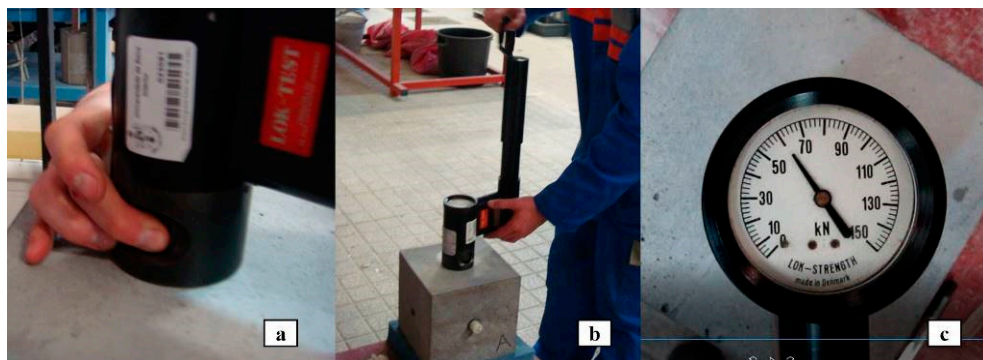
Figure 13. Pull-out test: (a) connection of the hydraulic jack, (b) loading, (c) reading.
