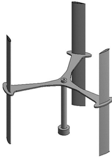
Figure 5. Straight bladed Darrieus turbine (or H-Darrieus), from [8]
