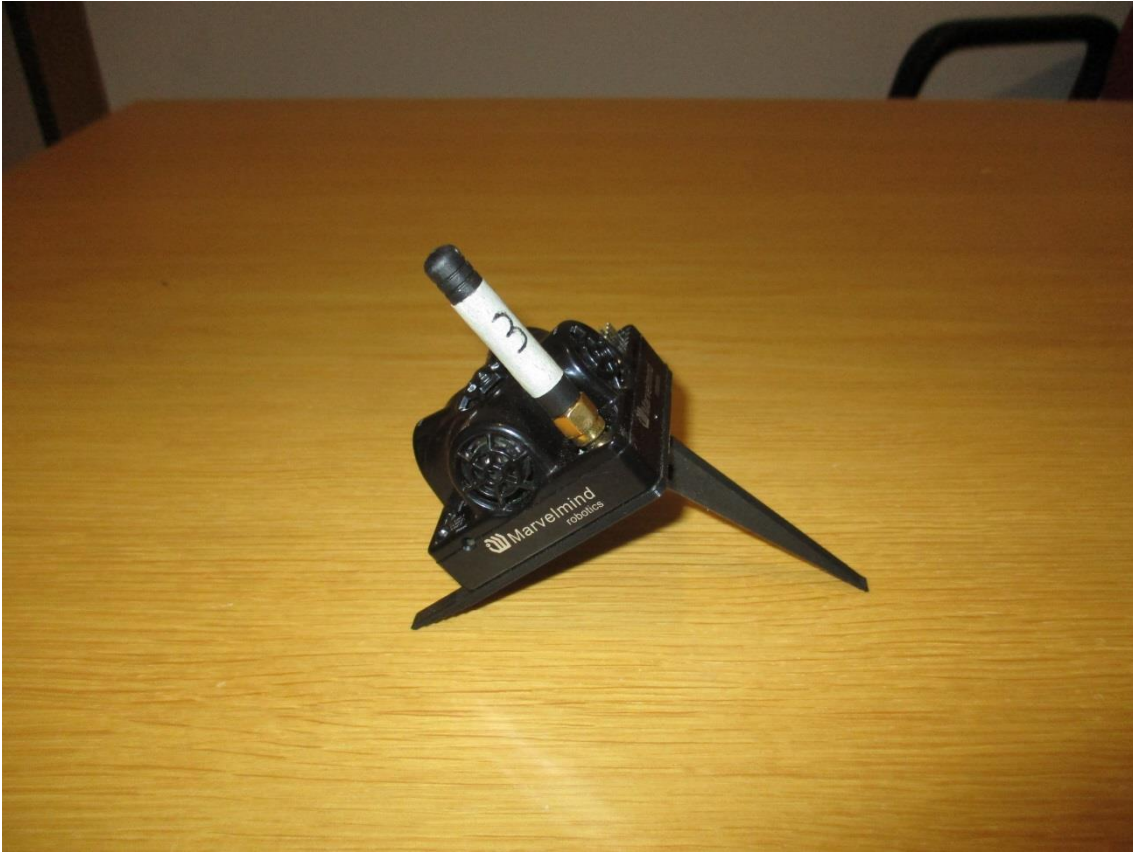
Figure 13 - Beacon mounted on a tripod with numbered label that matches the device address on the system
