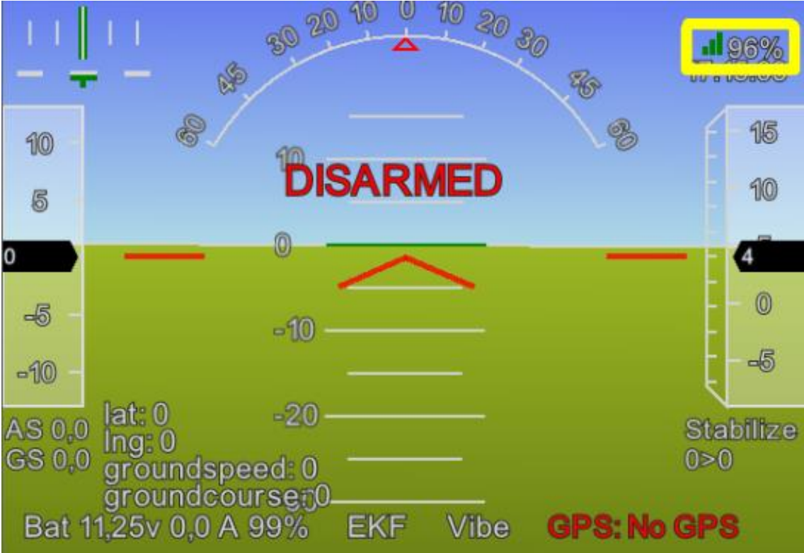
Figure 17 - Telemetry with 96% signal strength
