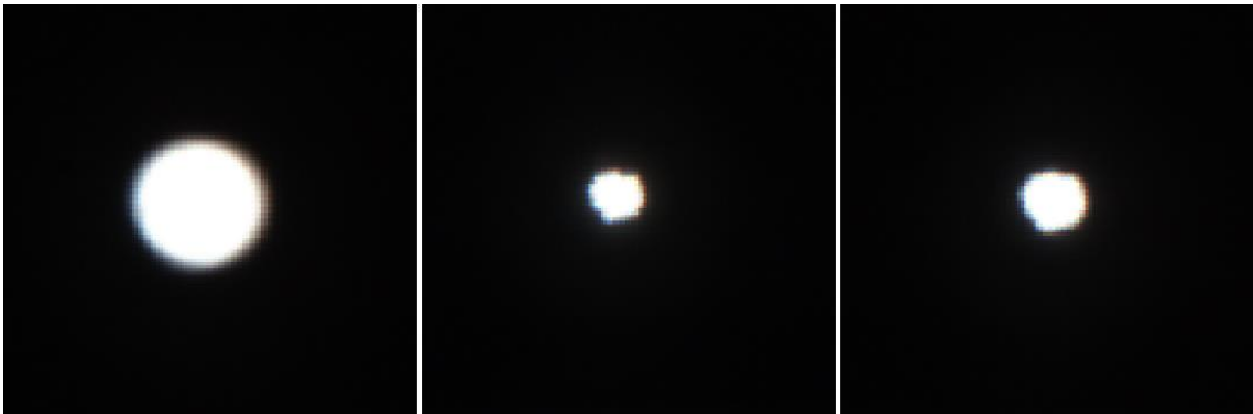
Figure 29 - Rotating the lens from very unfocused to most focused to ideally focused
