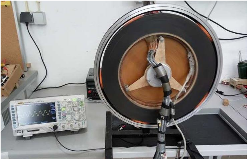
Figure 52 - No load current measurement
