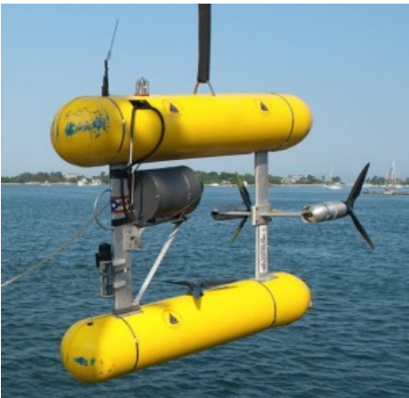
Figure 1.3: Seabed AUV (adapted from [9]).
