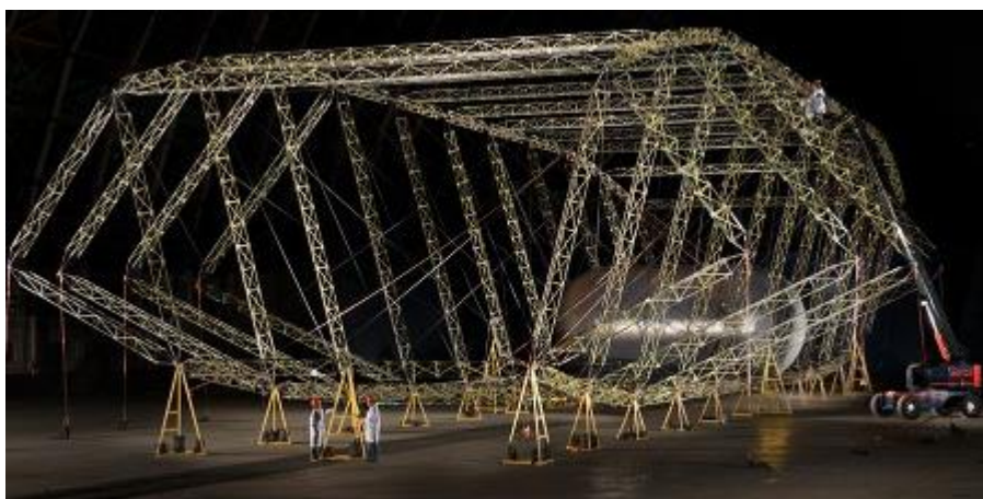
Figure 3 - Aeroscraft internal structure [13].
