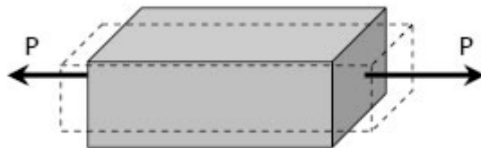
Figure 11 - Part under tensile stress [32].
