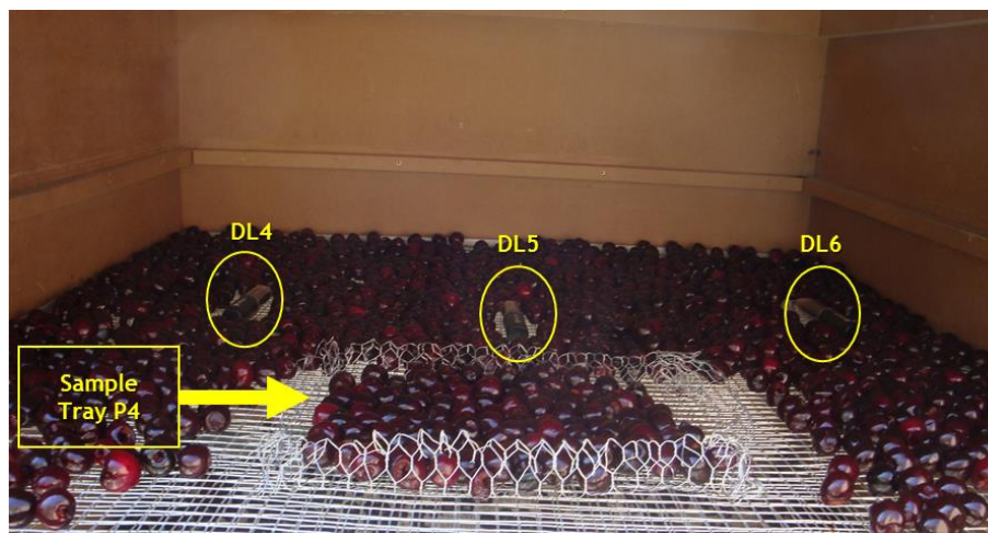
Figure 2 - Disposition of data-loggers DL4, DL5, DL6 on tray located on position P4 and sample made of malleable aluminum mesh
