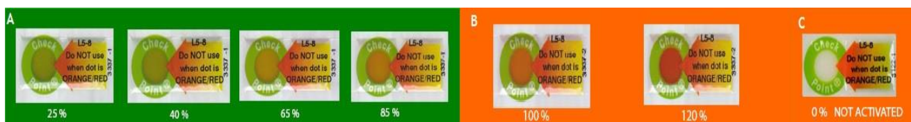
Figure 2. Illustration of the hydrolysis process of CheckPoint®. a) Primary TTI color state (green); b) Red-orange states, which indicates that the product is not fit to be consumed; c) TTI has a white coloration, which means that it has not been activated and cannot monitor the product's conservation status [26].
