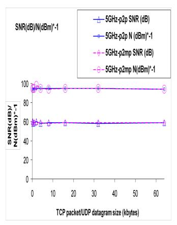
Fig. 2- Typical SNR (dB) and N (dBm). WPA links.
