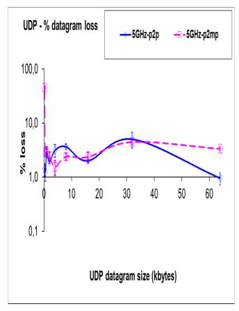
Fig. 6- UDP – percentage datagram loss versus UDP datagram size. WPA links. Log scale.
