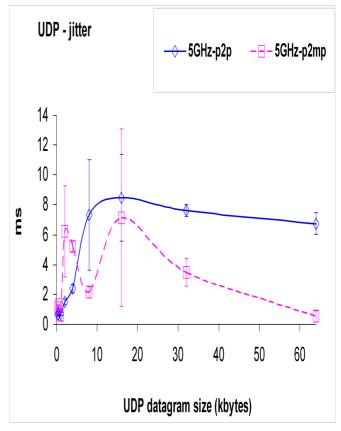
Fig. 4- UDP - jitter versus UDP datagram size. WPA links.
