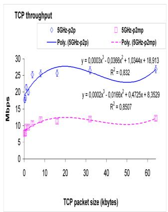
Fig.3- TCP throughput (y) versus TCP packet size (x). WPA links.
