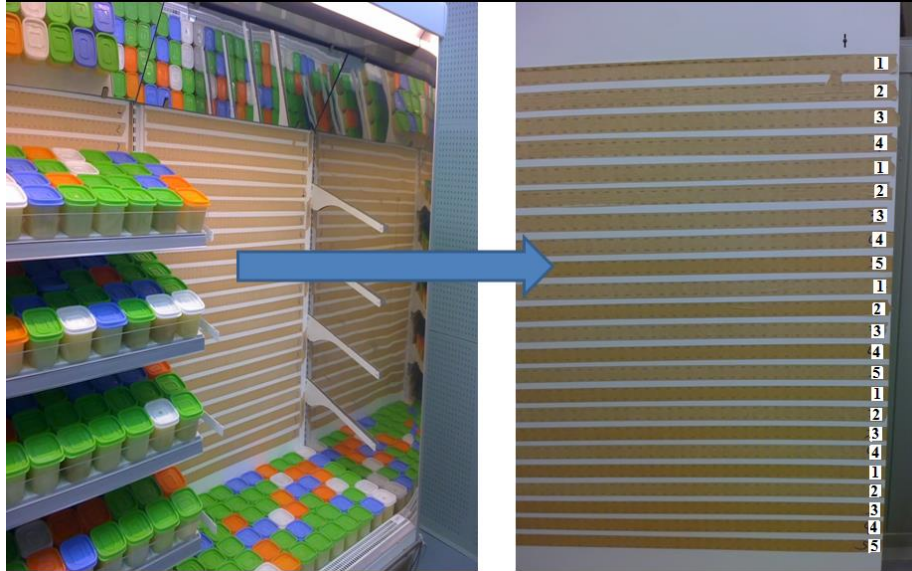
Figure 4: VORDC with PBP completely closed.
