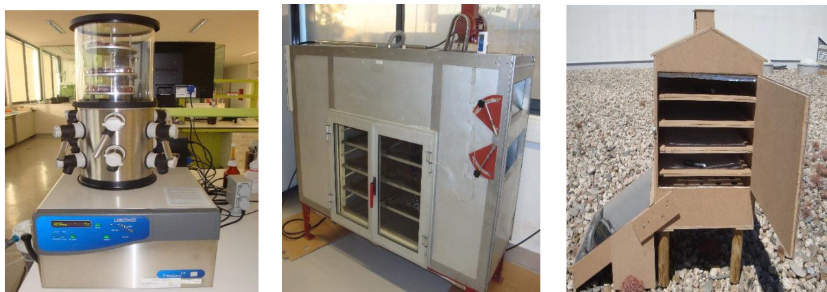
Figure 1. Images of dryers: lyophilizer (left); hot air (center) and solar (right)
