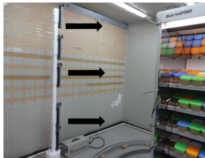
Figure 5. Location of centrifugal fans used to provide auxiliary ventilation.
