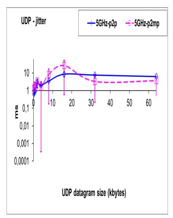
Fig. 5- UDP - jitter versus UDP datagram size. WEP links. Log scale
