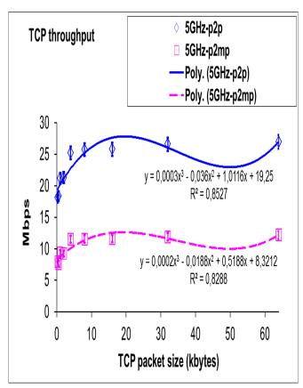
Fig.3- TCP throughput (y) versus TCP packet size (x). WEP links.
