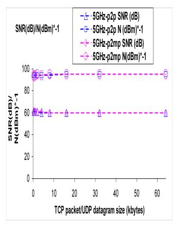
Fig. 2- Typical SNR (dB) and N (dBm). WEP links.
