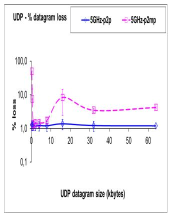
Fig. 7- UDP – percentage datagram loss versus UDP datagram size. WEP links. Log scale.
