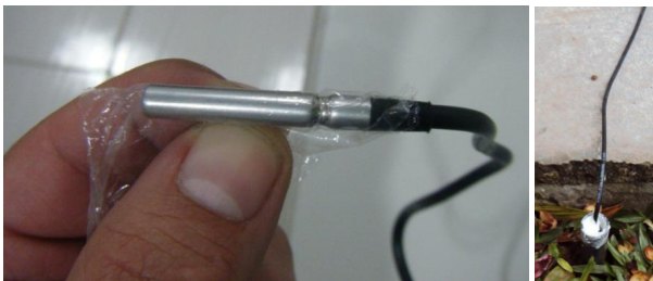
Figure 3: Sensor (left) and sensor-tube assembly inserted in the soil.
