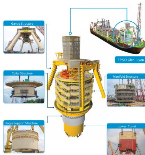
Figure 2.13: Turret schematic (image from ref. [21])
