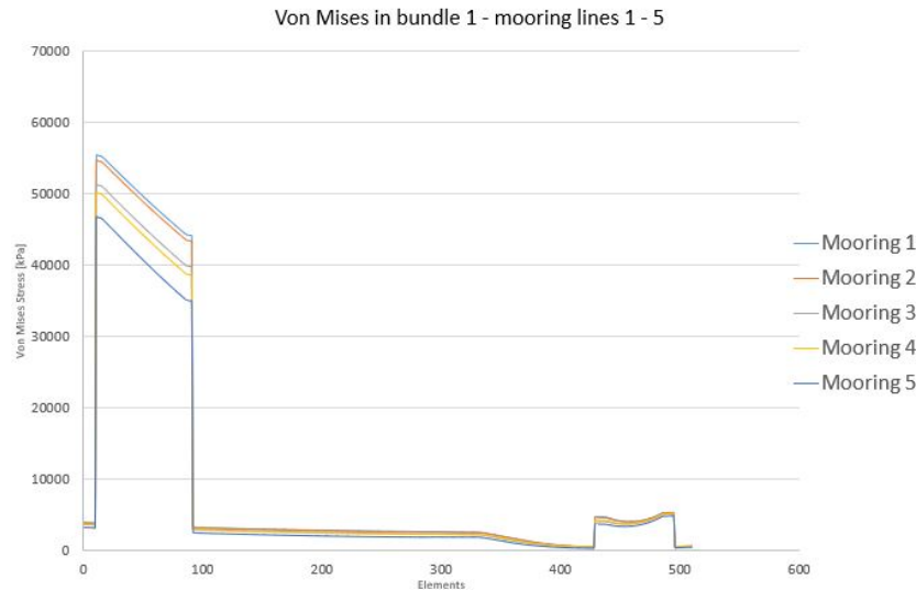
Figure 4.14: Von Mises stress - Bundle 1
