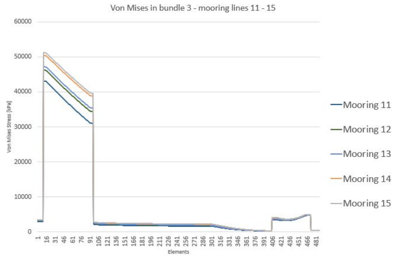
Figure 4.16: Von Mises stress - Bundle 3
